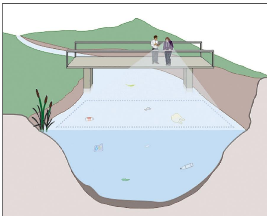
Figure 15: Illustration of a visual observation assessment of floating macroplastic debris. Source: Adapted from Hurley et al. (2023).
