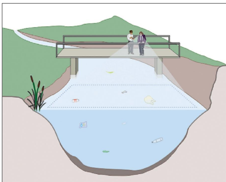
Figure 34: Illustration of a visual observation assessment of floating macroplastic debris. Source: Adapted from Hurley et al. (2023)
